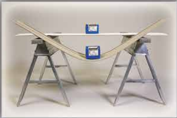
In strictly controlled laboratory comparisons, Charter Oak remained rigid, while the competition sagged.
